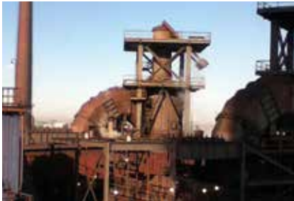
Every week this boiler is inspected with a thermal imaging camera to monitor the condition of the refractory lining.
