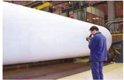
Inspection of the moisture distribution in the paper web shooting past at a speed of 1600 metres per minute.
