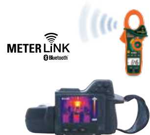
Thanks to MeterLink, the values read by the clamp meter are displayed on the thermal image.
