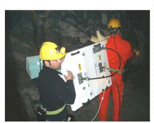
RIS Configuration with 80 MHz Shielded Antenna- Acquisition Phase
