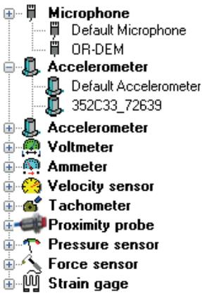
OROS 3-Series analyzers are designed to handle numerous transducer types without additional gears. Inputs are compatible with:
