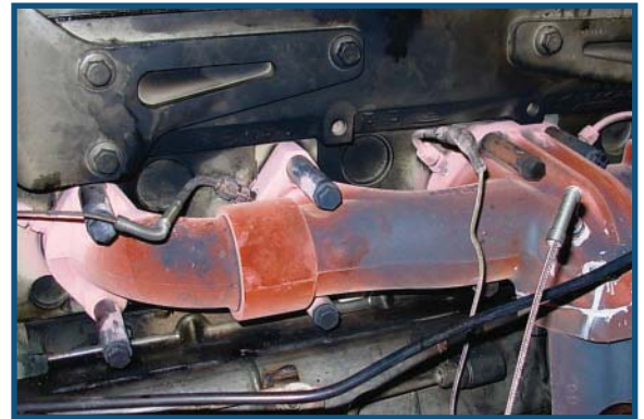
Hot Exhaust Manifold Under Test
