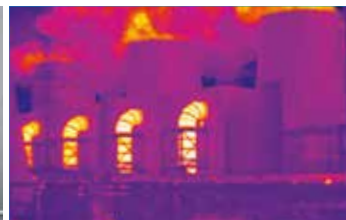
Heat leakage in a steam installation due to insufficient insulation.
