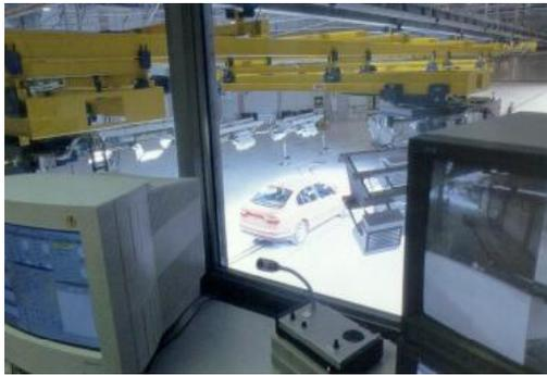
The use of high speed photography and videography achieves an essential contribution for the collection of relevant data at automotive safety testing. Today especially the high-speed video systems are gaining on importance.
