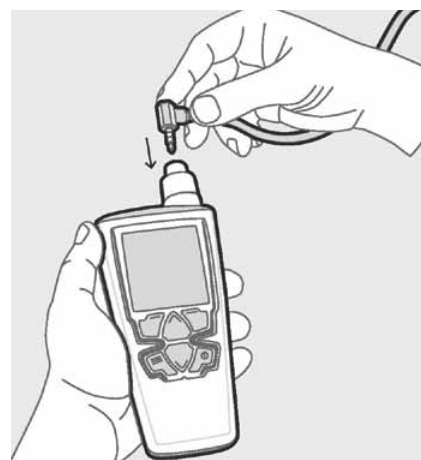
Snapping a connector to the indicator HM40 to read the measurement results.
