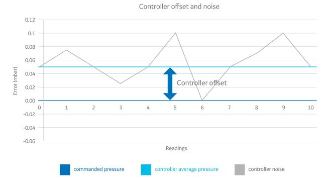
**Figure 7:** Controller offset and noise.
