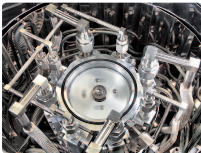
Rotating substrate holder surrounded by eight linear gas nozzles.
