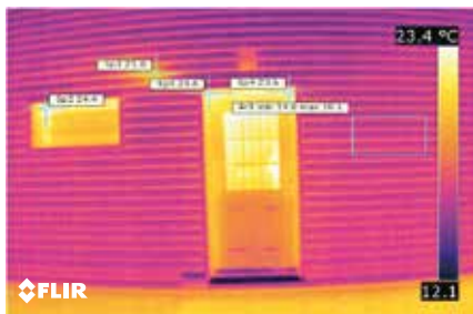
These thermal images show heat leakages from the vented hood and from the lintels of the windows and doors in both the heated and in the non-heated apartments. Room and door insulation was consequently improved.
