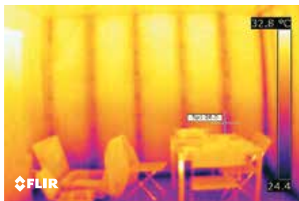
This thermal image shows that the bearing profiles in the indoor partition wall contribute to thermal bridges between the apartments. The new prototype therefore had improved indoor partition wall insulation.
