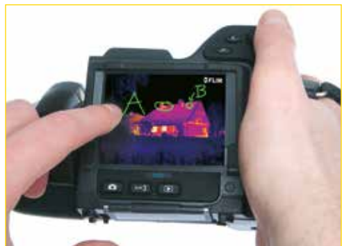
Thermal image of the same building, now using the MSX-setting. Note that more details are visible, making it easy to locate ventilation grids and see brick structure.
