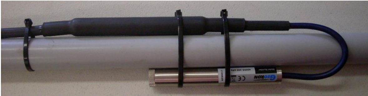
Figure 4.1: SAAPZ mounted to PVC conduit.
