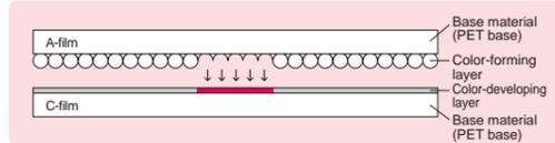
**Mono-sheet type** medium pressure, high pressure, super high pressure (3 types)
