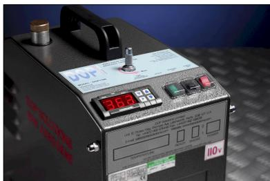
The vernier control is located immediately in front of the carry handle. Turning the vernier anti-clockwise allows more oil into the heat exchanger and thus increasing aerosol output. The vernier is
