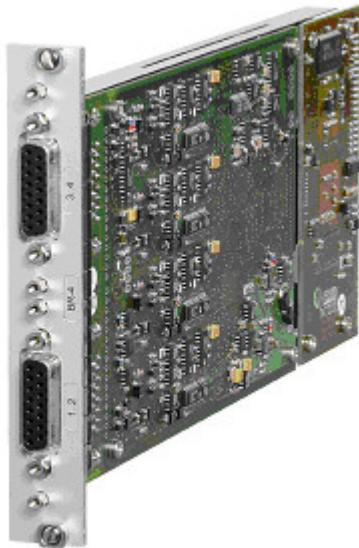
The **BR4** is an all-purpose bridge amplifier for 4 channels (also employable as a DC differential amplifier) available as a modular plug-in for the imc CRONOS-PL and as a configuration module for CRONOS-SL. It enables measurement of four measurement bridges or strain gauges which are excited with your choice of either DC or CF.
