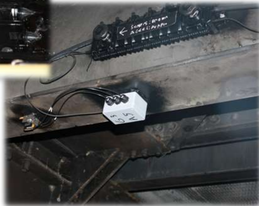
Main cable feed tapping point and industrial grade IP69 splice tray. (below)
