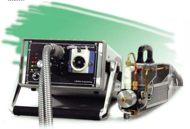
The Rotating Disk Thermodiluter accessory allows you to dilute the sample at the point of measurement. This preserves the size distribution and concentration so that particles are measured properly by the EEPS spectrometer. Dilution temperatures are selectable, enabling you to study volatile or semivolatile fractions.
