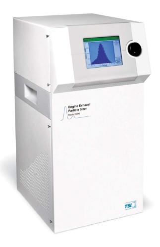
The Engine Exhaust Particle Sizer™ (EEPS™) spectrometer is a fast-response, high-resolution instrument that measures very low particle number concentrations in diluted exhaust. It offers the fastest time resolution available—10 times per second—which makes it well-suited for dynamic and transient tests. It measures the size distribution and number concentration of engine exhaust particle emissions in the range from 5.6 to 560 nanometers, covering the entire range of interest.
