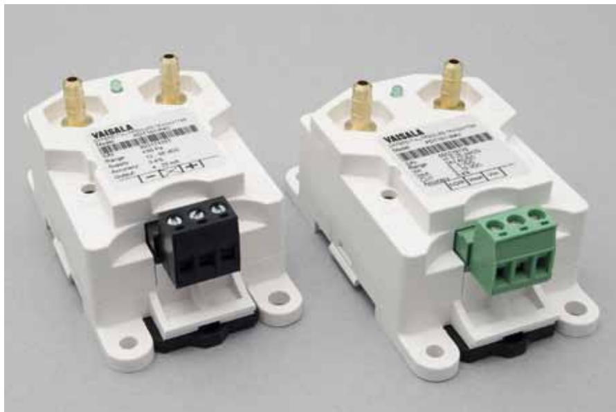
Vaisala Differential Pressure Transmitter PDT101 with current output (black) and voltage output (green).
