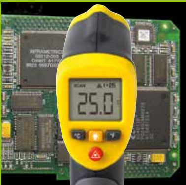
IR thermometer, measures temperature in one point.
