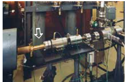
During an oxygen pressure shock test, the material in the container is exposed to a rapid pressure rise.
