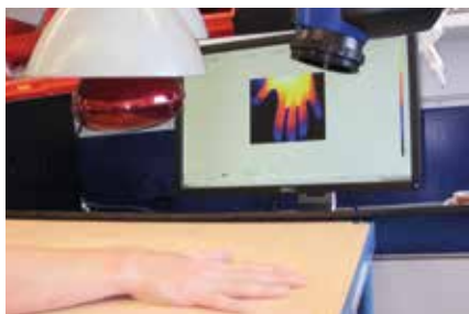
The IR lamp delivers a thermal stimulus to the skin. The thermoregulatory response is then recorded using the thermal imaging camera.
