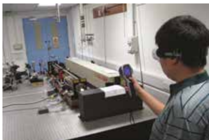
Research assistant Yong Ma demonstrates the use of the FLIR thermal imaging camera in the laser room.
