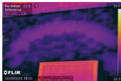
Below the surface of this wall along the nave contains arches for better weight distribution.
