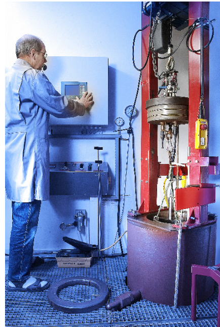
High pressure test tank. Pressure range up to 700 bar.
