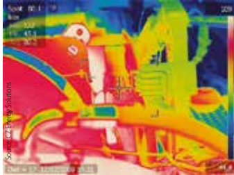
A thermal imaging wind turbine transmission survey. This survey was performed at a height of around 50 meters.
