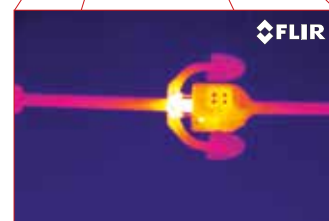
Thermal image of a high voltage installation taken from a longer distance still allows you to see all details.
