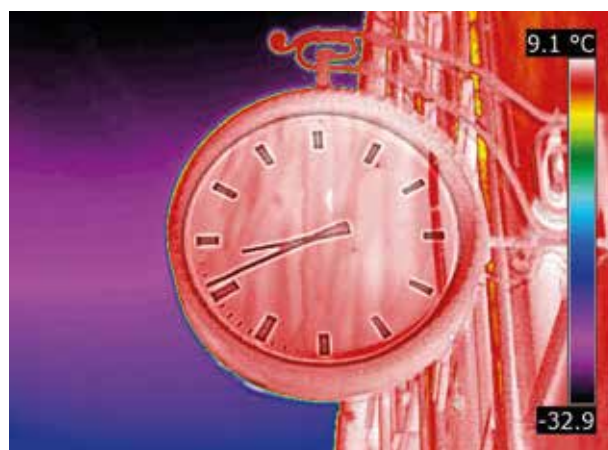
Thermal image with MSX®: Although glass is not transparent for infrared radiation this thermal image clearly shows the hands of the clock behind the glass. This is only possible thanks to MSX® technology that overlays a part of the visual image over the thermal image. The result: thermal images on which the smallest details can be seen.
