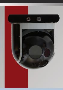
Combining the benefits of three unique sensors into a small Triple Camera platform including IR, UV, and TV.
