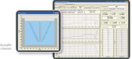
Sample flow and velocity profile collected in a rectangle channel.
