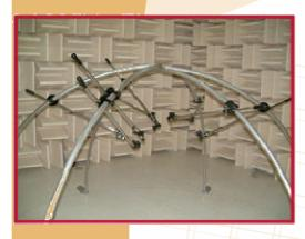
To make an easy job of sound power measurement according to ISO3741 in reverberant room, ISO3744 in normal rooms, ISO3745 in semi anechoic and anechoic environment, ISO3746 in external open space, our PRO-250 12ch system offers the ideal turn-key solution:
