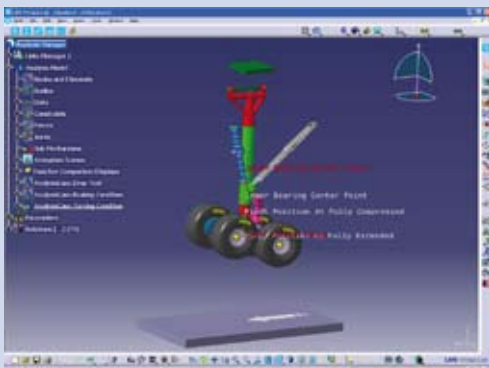
Various components can be modeled flexible increasing simulation accuracy.
