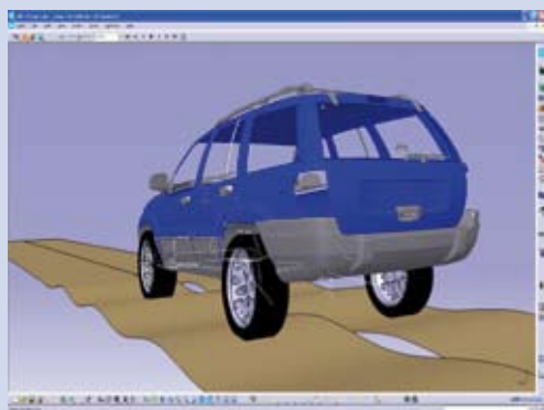
Vehicle simulated driving on a flat, or uneven 2 or 3D road including a digitized proving ground.
