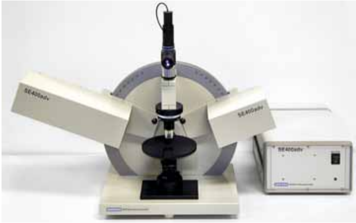
Laser ellipsometer SE 400adv with controller
