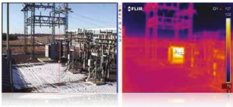
Figure 10. Visible light and IR images of a substation showing a transformer with excessive temperature.
