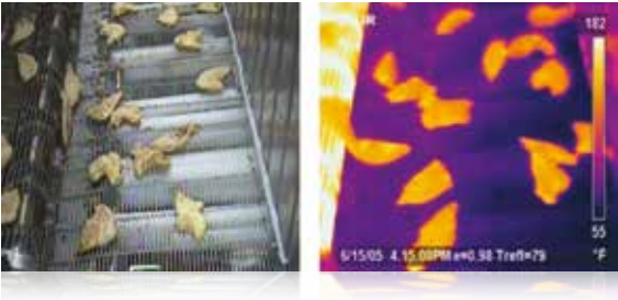
Figure 6. An IR temperature measurement and thermographic image are used to locate undercooked chicken tenders and stop the line so bad parts can be removed.
