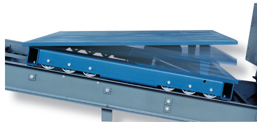
Platform Articulates for Specimen Loading and Unloading
