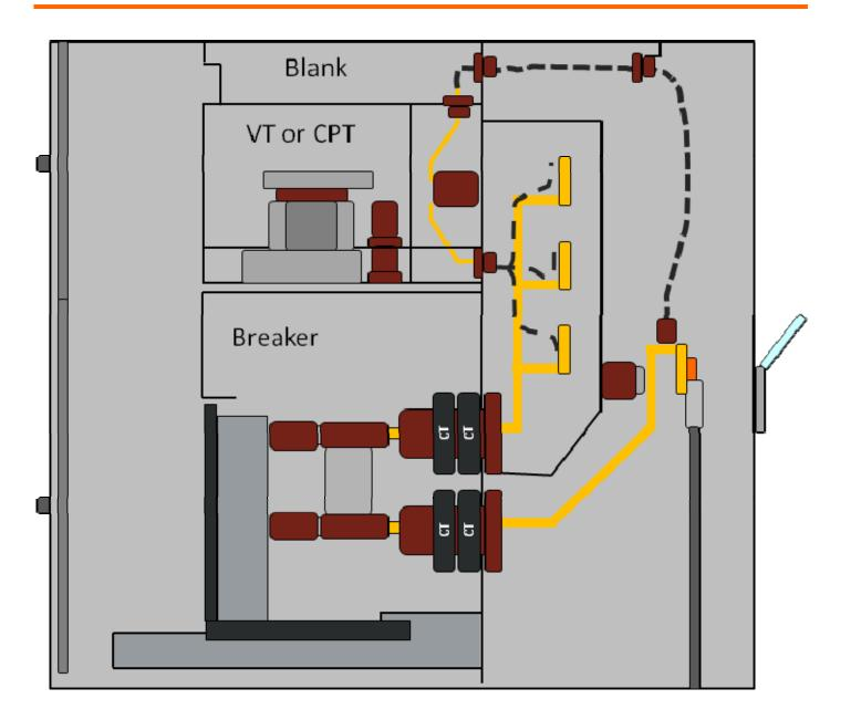
Non arc-resistant equipment is far more common. Most older equipment is not arc-resistant and secondary equipment such as motor terminal boxes and transformers are almost never arc-resistant. Non arc-resistant is not designed to "resist" an electric arc and will catastrophically fail under an arc-fault condition.
