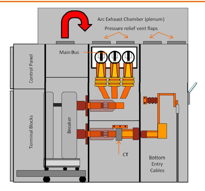
There are two types of switchgear—arc resistant and non-arc resistant.
