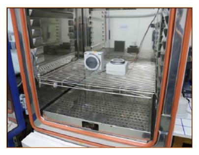
Humidity testing confirms no degradation of device due to increased levels of relative humidity.
