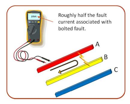
Then there is an arcing fault. This is shown by a High impedance short circuit, a "Low" current and a powerful explosion.
