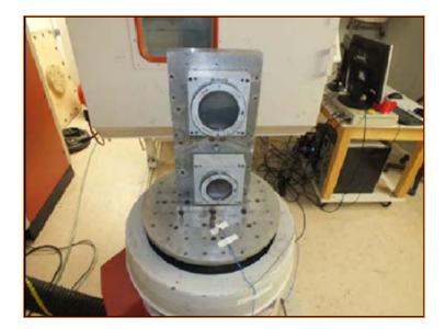
Vibration testing confirms the device does not disintegrate during severe ongoing vibrations as found in marine engine rooms.
