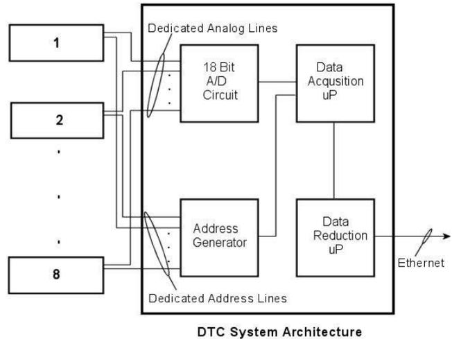
**DTC Initium Mainframe Architecture**
