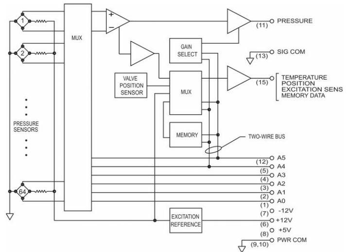
Another advanced feature is the ability to derange the ESP scanner upon command. This alters the gain on the amplifier to derange the scanner by a factor of three, enabling additional wind tunnel tests to be conducted without re-instrumenting the model with lower range ESP scanners. To optimize the accuracy of the DTC scanner at the highest gain, the optional dual range calibration is recommended.
