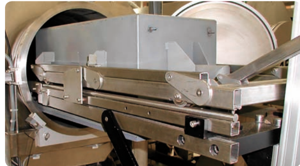
P400A with reaction chamber in loading position.
