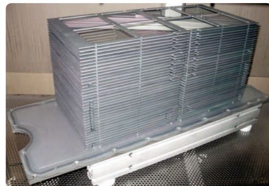
Deposition cycle times from 2 to 4 seconds are possible for both large surface areas (left) and large volume batches (right). The substrate size to the left is 600 × 1200 (mm). The number of substrates to the right is 288 pcs.
