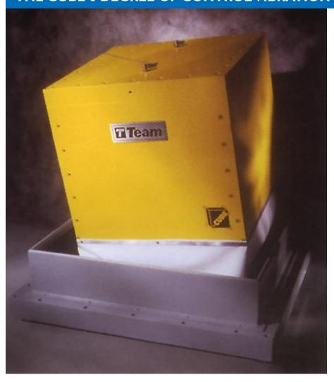
EAM Corporation is taking 6 degree of freedom testing a giant step forward. An advanced technology hydraulic test system that offers 6 Degrees of Control™, the CUBE™ can accurately replicate virtually any vibration environment, including very high frequencies, with precise digital control.
