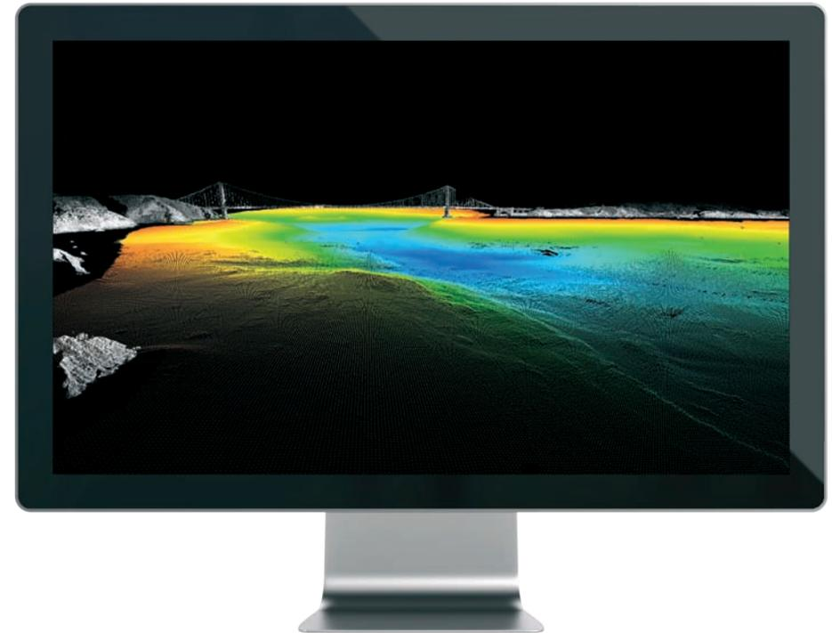
The LiDAR Point Cloud Generator Module in POSPac MMS is used to combine the raw Lidar range measurements with the navigation data to generate point cloud data as above.
