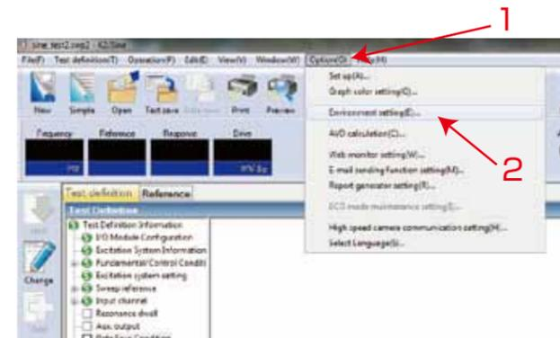
Figure 2: Opening the Digital I/O Setup
