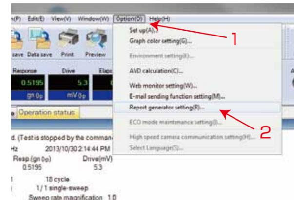
Figure 1: Open the Report Generator Setup
