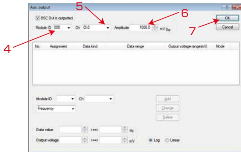
Figure 3: Configuration of the OSC output
