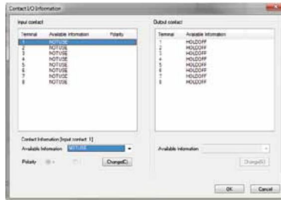
Figure 5: Digital I/O configuration menu
