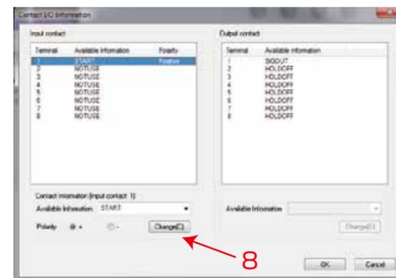
Figure 7: Configure the digital I/O
