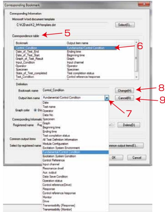
Figure 4: Linking the test results
