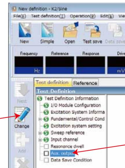
Figure 1: Open the Auxiliary Output Setup
