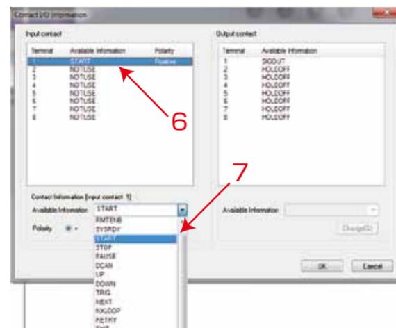
Figure 6: Configure the digital I/Os
