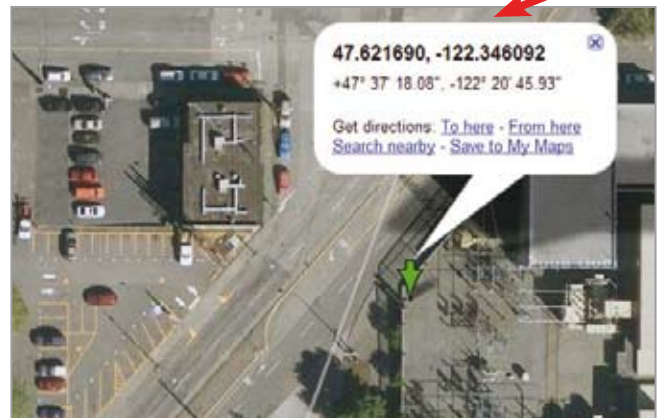
Reporter 8.5 supports the embedded GPS feature in FLIR's P660, B660, and SC660 cameras. Downloaded images contain GPS coordinates. By clicking the icon, you can see a satellite image, get address information, even street directions to add to your report if needed. (The green arrow shows the FLIR camera position).
