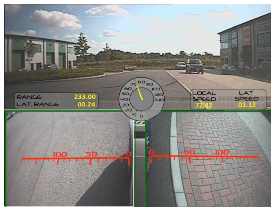
Left: Example screenshot of a Vehicle Separation Application, using two cameras.
