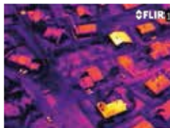
The buildings with yellow colored roofs show there is a moisture or insulation problem.
