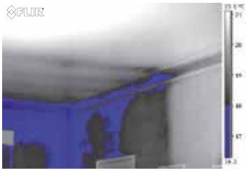
The relative humidity alarm alerts you to the areas where there is a risk of condensation. In the image below the area at risk is indicated as blue color.
