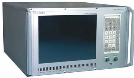
Fig.3 Omnisens DiTeSt Analyzer for distributed temperature and strain measurement in optical fibers
