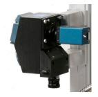
tivity and dynamic range. A design-optimized objective lens comes with each Starter Kit, providing excellent chromatic compensation and imaging results over the 250nm-600nm UV-VIS spectral range. The 28mm focal-length lens provided with the Hyperspec UV Starter Kit has been optimized for high resolution of UV wavelengths.
