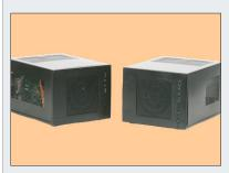
Headwall's Hyperspec Data Processing Unit (HDPU) comprises a high-performance CPU and GPU combination plus high-capacity storage to provide instantaneous management of hyperspectral image data
