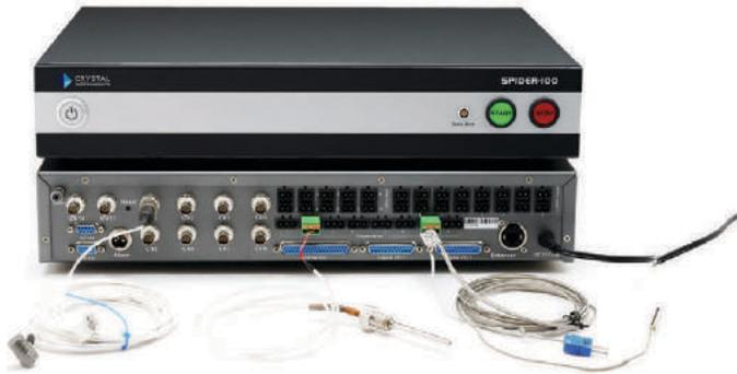
The Spider-100 Temperature, Humidity, & Vibration Controller
