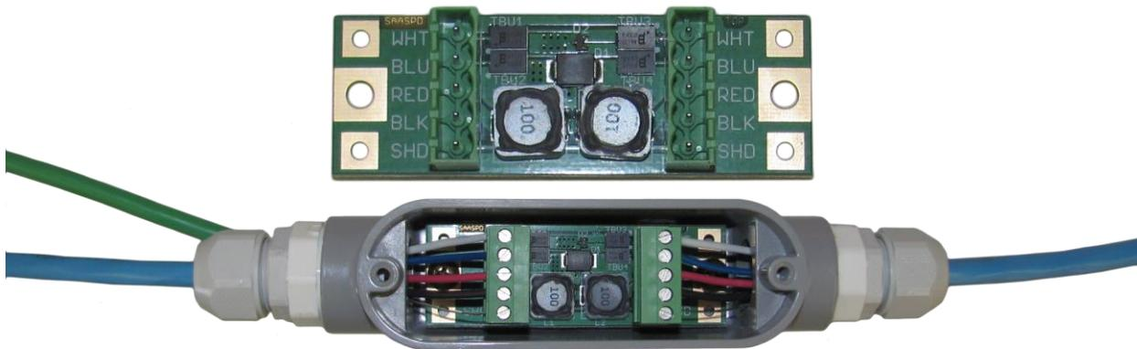
Figure 1.1 SAASPD board and housing.
