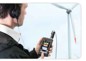
The integrated GPS receiver and the optionally available GPS antenna record the location and the time of your measurements. Additional documentation of data can be accomplished by connecting a USB camera and making simultaneous video recordings. Thus, SQobold provides innumerable possibilities from noise mapping to comprehensively documented test runs.
