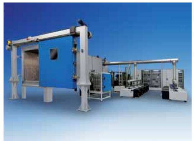
24 cu.mt chamber for temperature, humidity and altitude tests, characterized by fast depressurization from ambient down to 45 mbar in 1 min. Special standard requested: DEF STAN 00-35 CL9 severities B C Y E.
