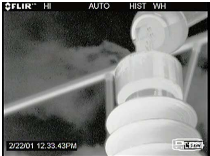
SF6 leak from a high voltage insulator
