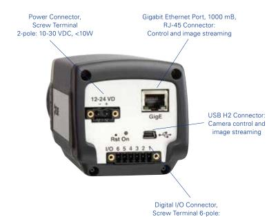
Digital Out: 2 outputs, opto-isolated, 10-30V supply, 100mA. Digital In: 2 inputs, opto-isolated, 10-30 V.
