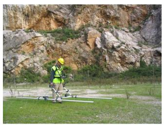
RIS Configuration with 25 MHz Unshielded Antenna- Acquisition Phase
