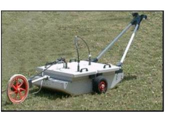
Separated transmitter and receiver antennas permit bistatic data collection (antennas can be spaced up to 1 meter apart).
