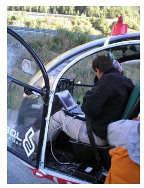
RIS Configuration with 100 MHz Shielded Antenna- Acquisition Phase
