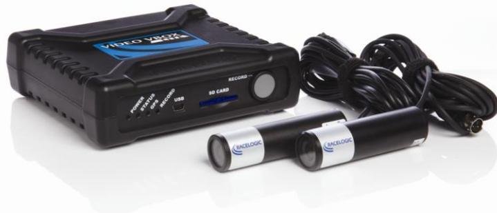
**Video VBOX Lite** takes the video captured from multiple waterproof cameras and combines it with a customisable graphic overlay, streaming the resulting video onto an SD card as a DVD quality MPEG4 file. A 10Hz GPS engine provides information such as circuit position, lap timing, speed (accurate to  $\pm 0.2$ km/h) and acceleration, whilst a single CAN channel can retrieve data such as RPM. CAN upgrades are also available to give a total of 2 or 4 channels.
