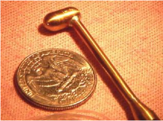
Five-Hole Embedded Sensor Probe for GE Aircraft Engines. Five Pressure Sensors are Contained in the Bullet-Shaped Tip
