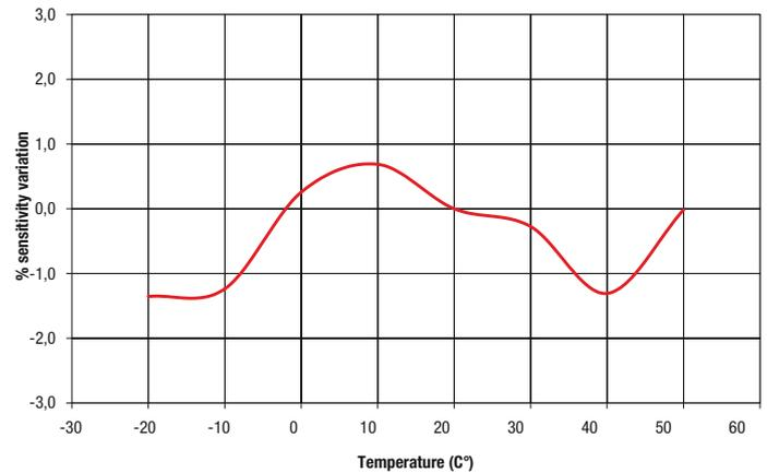
Graph 1: % variation of sensitivity of the LP PYRHE 16 pyrheliometer compared to the sensitivity at 20 °C, in the temperature range from -20 to 50°C.
